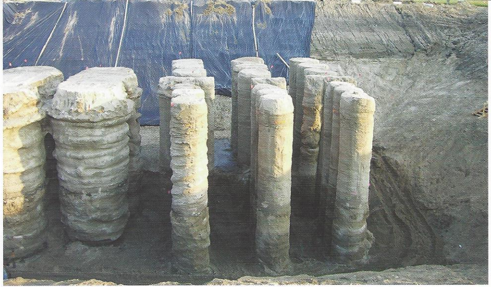
Landmark full-scale test of DMM techniques at Tuttle Creek, Kansas. The other four photos in this article are of the LPV-111 demonstration DMM project at Lake Ponchartrain, La., part of the USACE post-Katrina effort. This project remains by far the largest DMM application in the U.S., and one of the largest in the world. It set new standards in productivity and quality in North American Deep Mixing practice.
